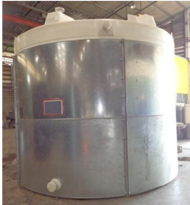
Hydrogen Peroxide 50% Storage Tank, 25m3
