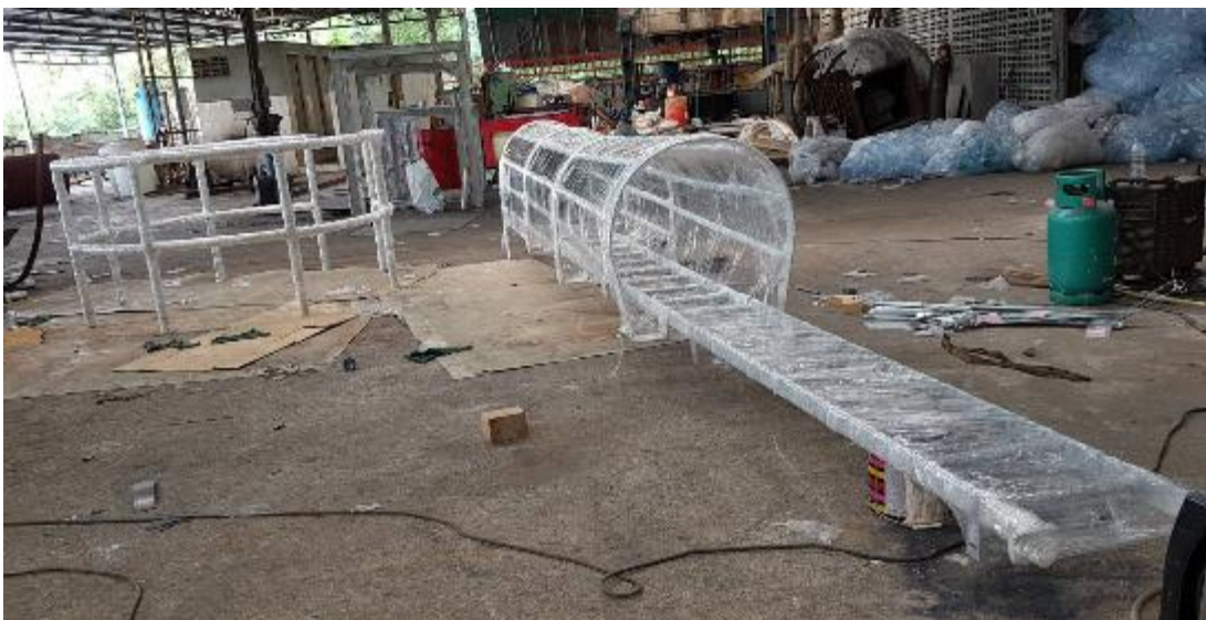
Hot-dip galvanized handrail and ladder with cage, 25m3
