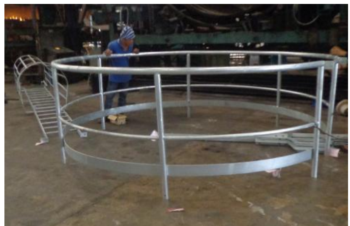
Hot-dip galvanized handrail and ladder with cage, 30m3
