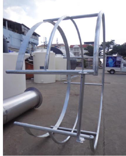
Hot-dip galvanized handrail and ladder with cage, 20m3 tank
