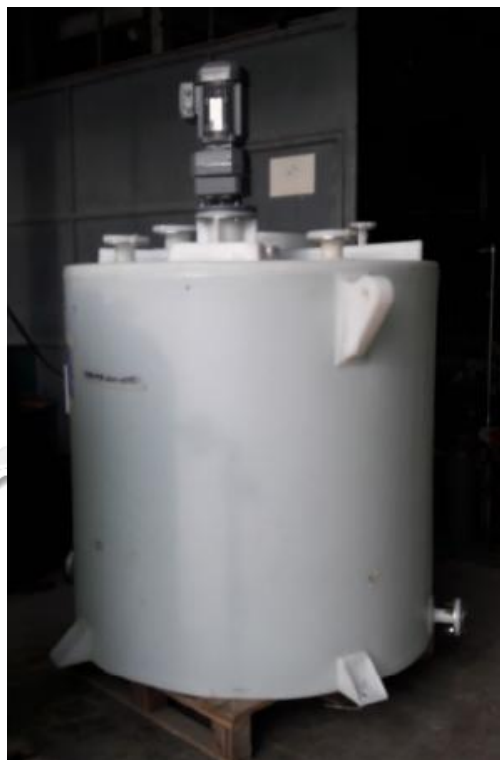
Preparation Tank - 1.5m3
