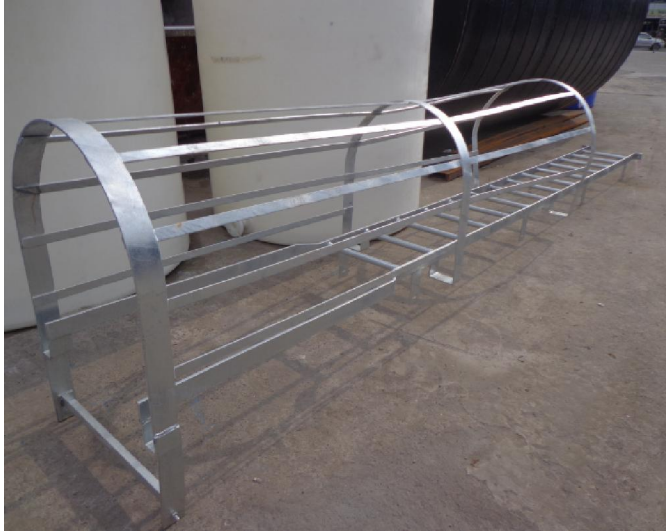
Hot-dip galvanized handrail and ladder with cage, 20m3 tank
