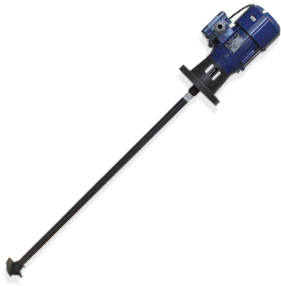
MIXVN/8 High speed mixer 1400 RPM. AISI shaft-PVC coated, different lengths available (630-730-830-930 mm). Marine impeller, diameter 70mm.
