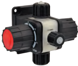
MF MULTIFUNCTION VALVE Multifunction valve (pressure, safety, antisiphon and bleed) 1/2" connections for different hoses diameters. FKM B or EPDM o-ring. PVDF body.
